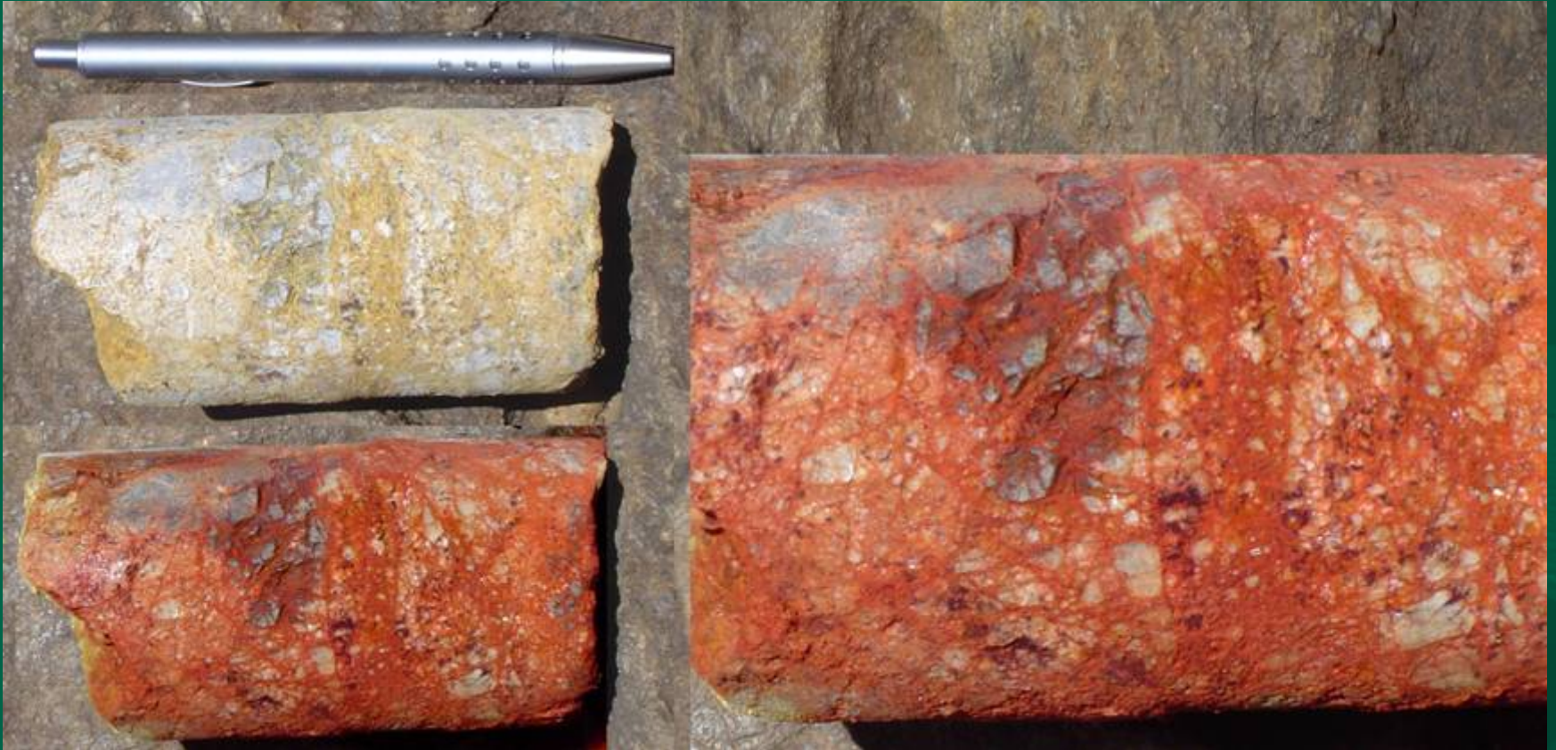
Drill Intersection showing “zinc zap” reaction
